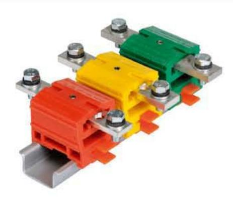
elmex offers a wide variety of Power / Bus-Bar / High Current Terminals suitable for all types of cables (solid, stranded, with fork type and ring type lugs) both in Polyamide 66 and Melamine Housing. In the Feed Through Range, Terminal types KUT25, 35, 50 and 95, with respective rated currents 101, 125, 150 and 232 Amps are available for connecting solid and stranded conductors.
